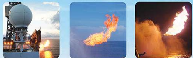
Fig. 5: Flaring gas at the DDKG-2 drill-ship during the testing main flow period of SYH-2; the DDKG-2 is some 86 m high above water and 42 m wide, the length of the gas flare is estimated at some 20 m long
