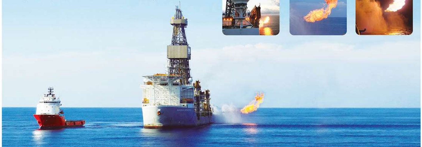
Fig. 5: Flaring gas at the DDKG-2 drill-ship during the testing main flow period of SYH-2; the DDKG-2 is some 86 m high above water and 42 m wide, the length of the gas flare is estimated at some 20 m long
