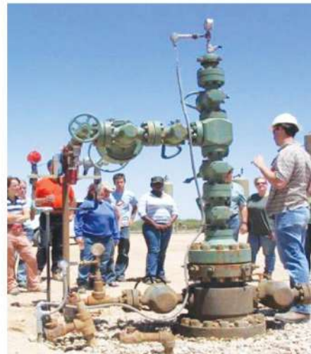
Fig. 1: Typical Christmas tree used on onshore wells or offshore platforms with dry (i.e. off the water) trees. (Source: oilandgasmanpowerprovider.blogspot.com)
