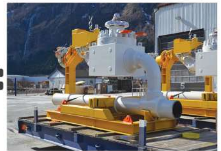
Fig. 7: Land vs deep-water pipeline crossing, a simple surface 16" pipeline tee (or T-crossing) is replaced with a massive subsea Inline Tee (ILT) (Source: gasprocessingnews.com and EAB Engineering)
