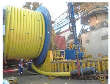
Fig. 5: Example umbilical manufactured as one continuous length and loaded onto multiple spools for transport and installation (Source: JDR and Oceaneering)
