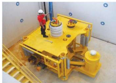
Fig. 2: Typical deep-water subsea Christmas trees (Source: Cameron/OneSubsea and GE/Baker Hughes)
