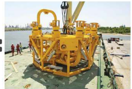
Fig. 8: Land vs deep-water manifold (Source: oilandgastechology.net and OneSubsea)
