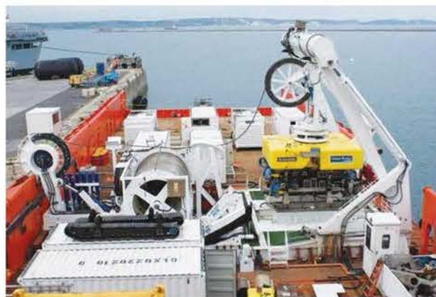
ROV installed on an installation vessel to support SIC operations
