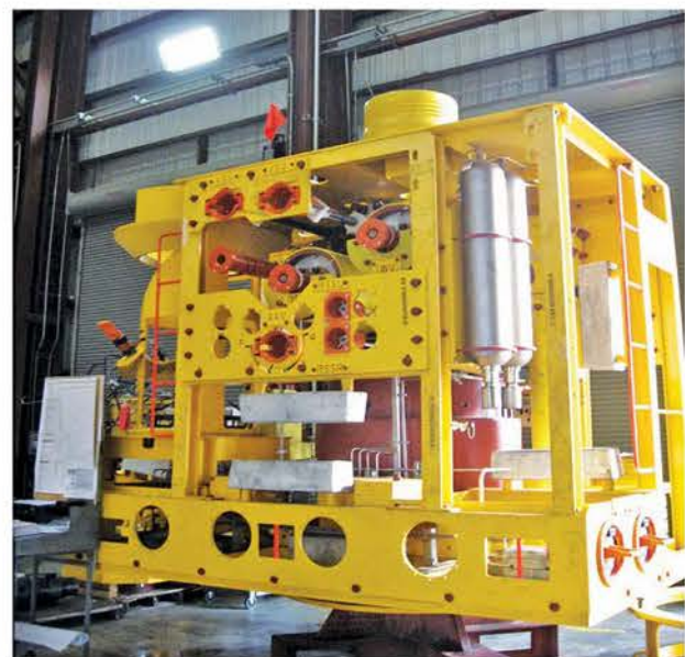
Typical Subsea Tree – designed for ROV compatibility
