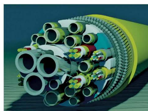
Cross section of typical umbilical – compliments of Quora
