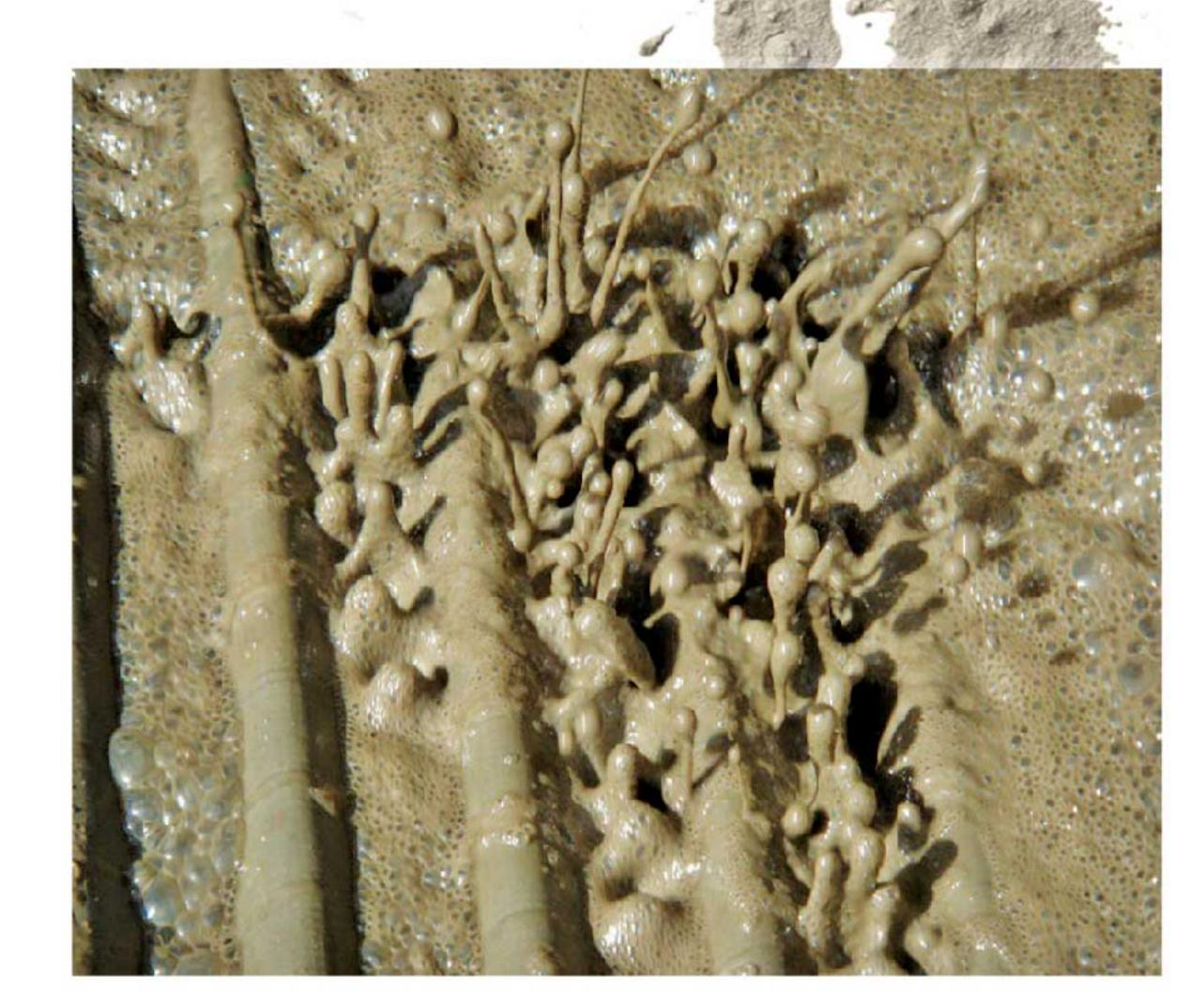
Beautiful bouncing mud on the shale shaker in action; the shale shaker is this vibrating sieve that separates drilling mud from rock cuttings
