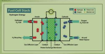
Fig. 4: Hydrogen Fuel Cells (Source Intelligent Energy)
