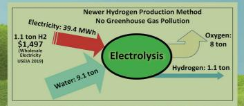
Fig. 3: Hydrogen Production by Electrolysis of Water (Wikipedia)
