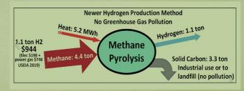
Fig. 2: Hydrogen Production by Natural Gas Pyrolysis (Wikipedia)
