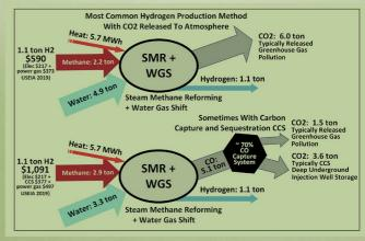
Fig. 1: Hydrogen Production by Natural Gas Reforming (Wikipedia)
