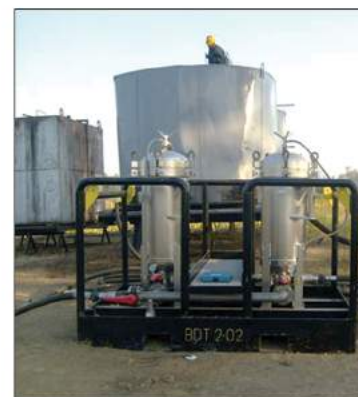
Fig 6: Filtration of formation water in Mann field before dumping into thirsty wells
